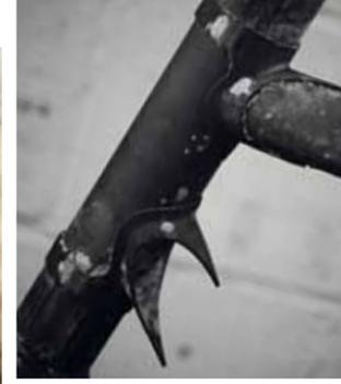
**Left** Headtube lugs have to be positioned precisely and require some persuasion
