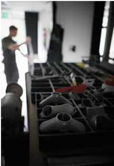
▶ First it's just the seat tube and bottom bracket and head tube, but soon we add the down tube and top tube, all having been mitred to fit just so. By Wednesday afternoon the main triangle is clamped up in the jig with head lugs and seat lugs in place and ready to be brazed.
