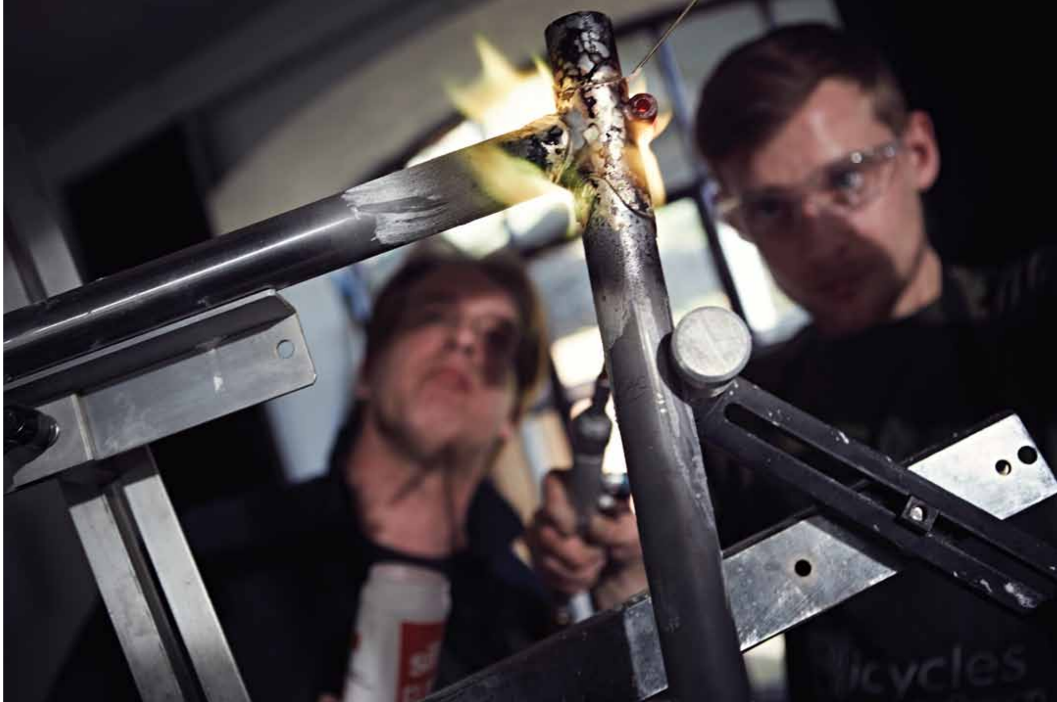
Above: Pete Bird keeps a careful watch as Cyclist brazes up the main triangle. For a beginner this can be slow, anxious work, heating the lugs with the brazing torch in one hand while feeding the thin rod of brass filler into the joint with the other
